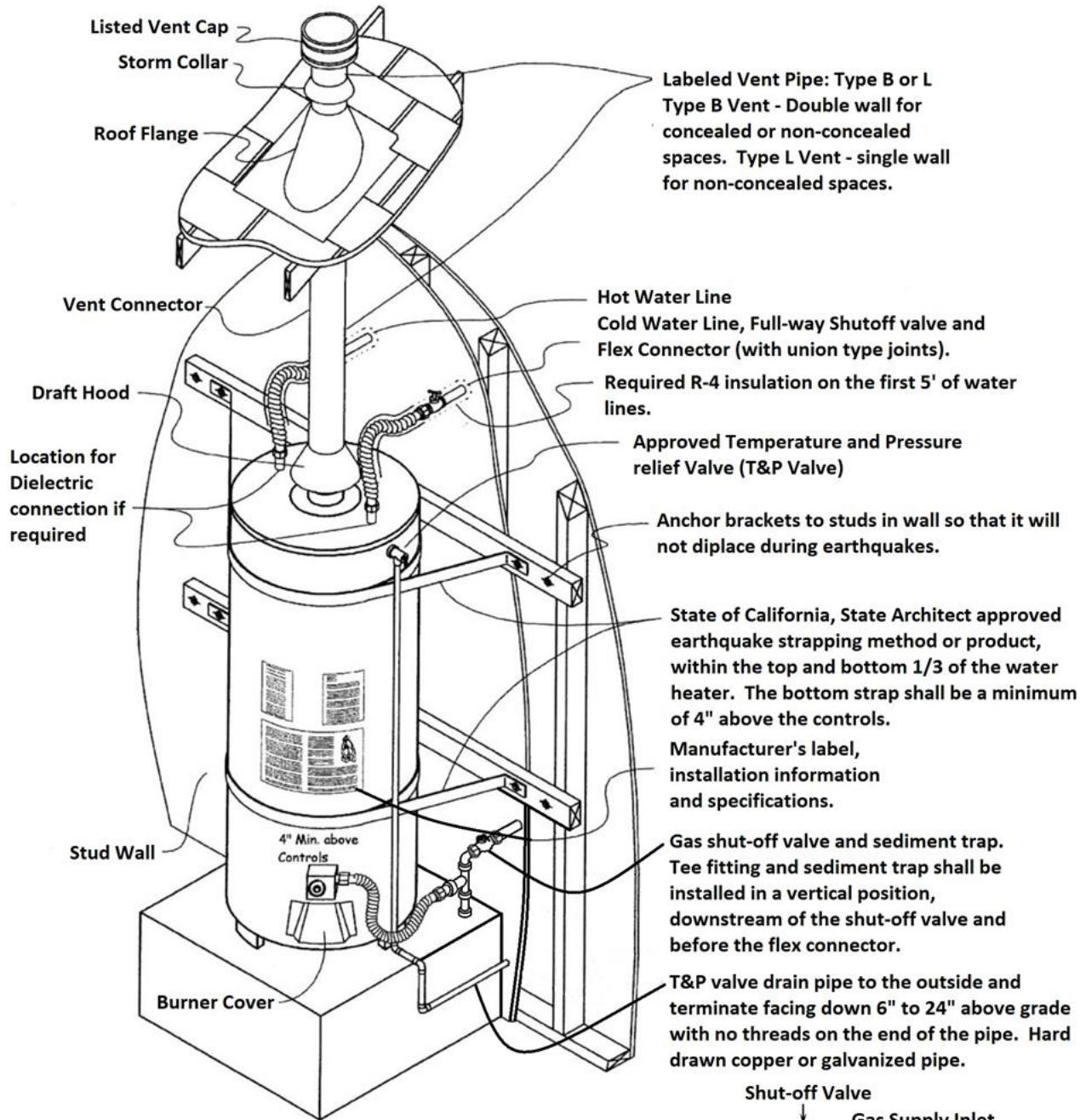
Appliances in garages shall be installed 18" above the floor to the burner-ignition device unless listed as flammable vapor ignition resistant (FVIR)
