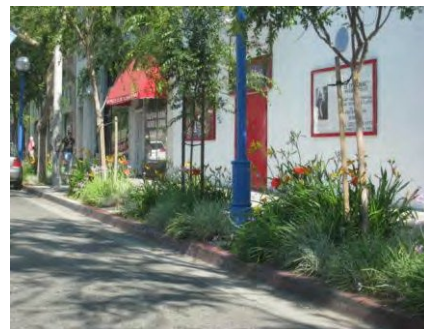
All continuous landscaped parkways collect stormwater runoff from the sidewalk
